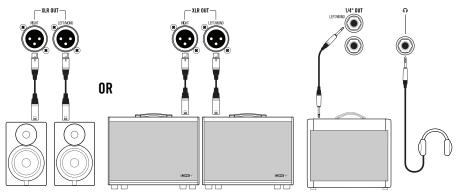
The Helix device's 1/4" and XLR output levels must be set to match your playback system. If you're only using headphones, for now, skip to step 9.
