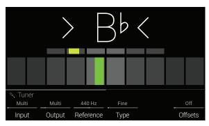
On Helix Control, hold the TAP footswitch until the Tuner screen appears:
