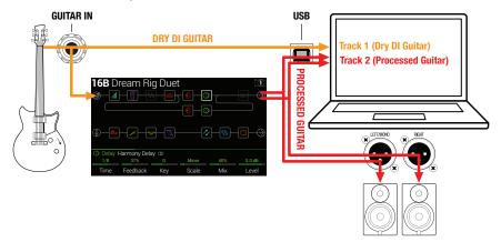
4. Set both tracks' outputs, as well as the DAW Master output, to Helix USB 1/2 to allow all tracks to play back through Helix.
