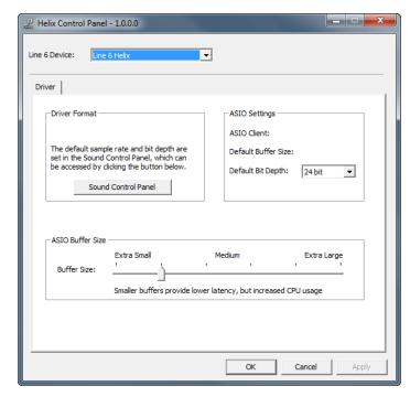
Sound This button launches the Windows Sound Control Panel, which is **Control** where you can optionally configure Helix to be the audio playback Panel device for multimedia applications (such as Windows Media Player, iTunes apps). These settings are not relevant for your DAW software since these applications utilize the standard Windows driver.
