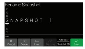
Move the joystick left or right to move the cursor. Snapshot names are limited to 10 characters.
