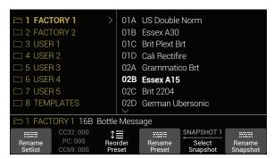
The dark text above Knob 2 displays the required MIDI messages for recalling the Helix device's setlists, presets, and/or snapshots from external MIDI devices or software. In the illustration above, the **FACTORY 1** setlist is recalled with a CC32 message of 000, the **02B Essex A15** preset is recalled with a PC (program change) message of 005, and **SNAPSHOT 1** is recalled with a CC69 message of 000.
