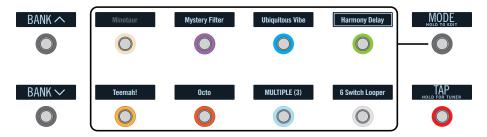
**NOTE:** If a switch is assigned to multiple blocks or items, its scribble strip reads "MULTIPLE (X)," where X is the number of assignments, and stepping on the switch turns them all on and off. If some blocks are on and some are bypassed, stepping on the switch toggles each block's bypass state.
